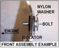
Carefully hold the Skid Plate up to the frame. Thread in the two RIMS bolts 4-5 turns and then thread the 6mm bolt, with washer, into the rear mount 4-5 turns.
